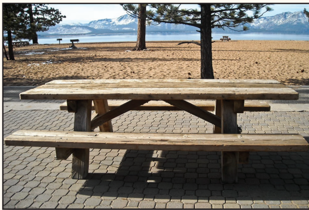
Figure 81—This picnic table at Nevada Beach day use area in the Lake Tahoe Basin Management Unit is a popular design that allows people who use wheelchairs to use either end without the appearance of “separate” space. A Forest Service shield is routed into the cross piece on each end, adding to the design appeal.
